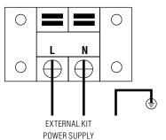
POWER SUPPLY VOLTAGE 220-240V AC WIRING SIZE 1.5mm<sup>2</sup>
