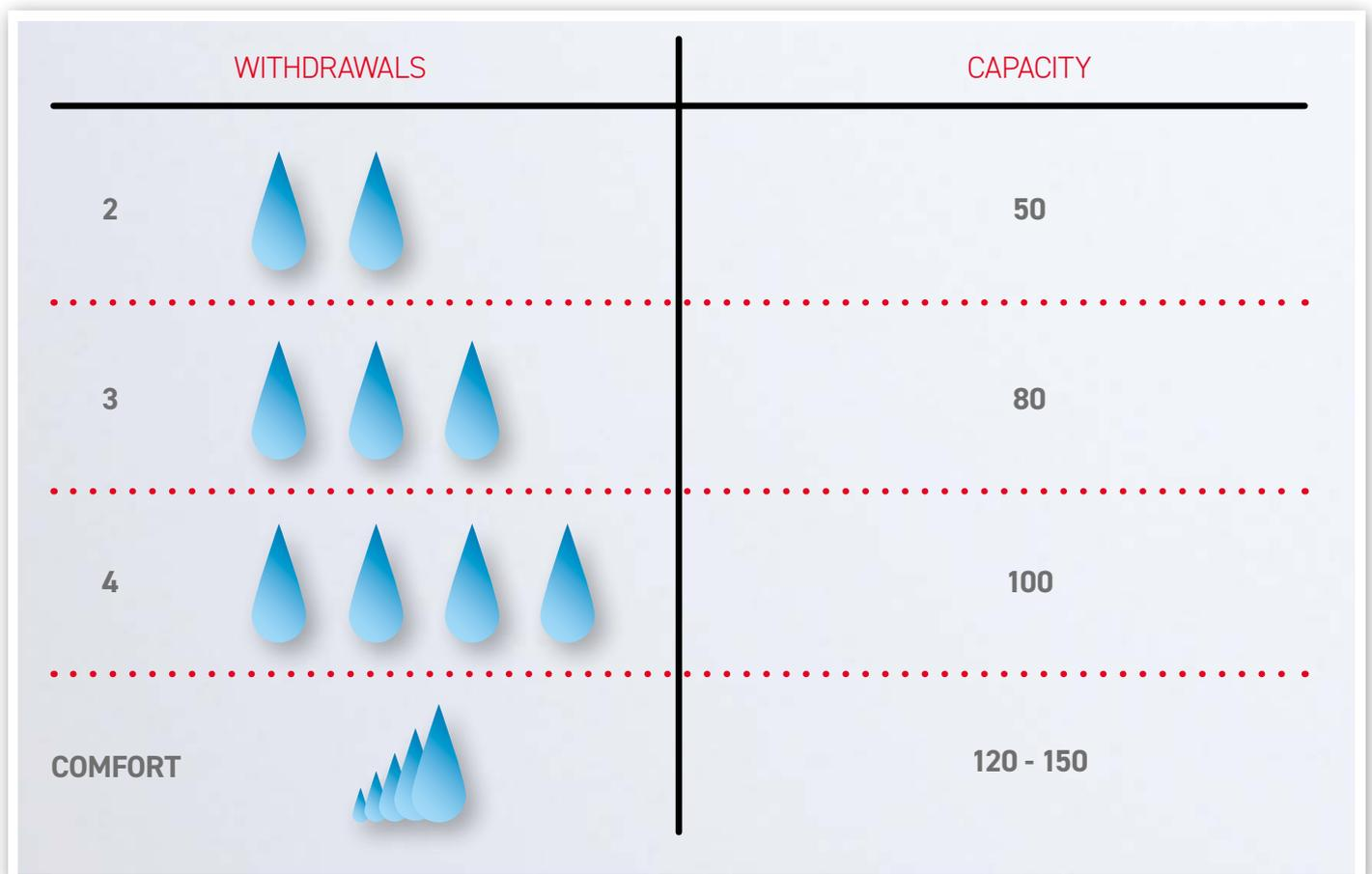
Simulation has been calculated considering 6 lts/min withdrawal mixed at 40°C for 6 minutes
