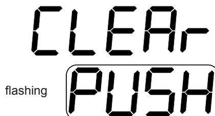
Pressing the key again during this display determines the reset of all meters relative to fuel consumption and the return to first stage fuel consumption display.
