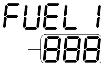
Press key **i** to access the PARAMETER VALUE MODIFICATION mode, during which the value of the parameter displayed flashes.
