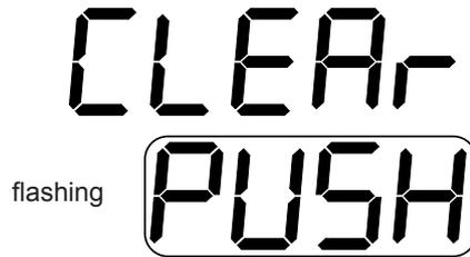
Pressing the key again during this display determines the reset of all meters relative to the functioning hours and the return to first stage functioning hours display.
