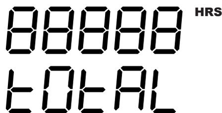
To reset all counters relative to fuel consumption, press the key i during the following display:
