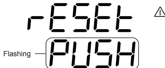
Pressing key R again causes the release of the appliance and the return to normal display mode.
