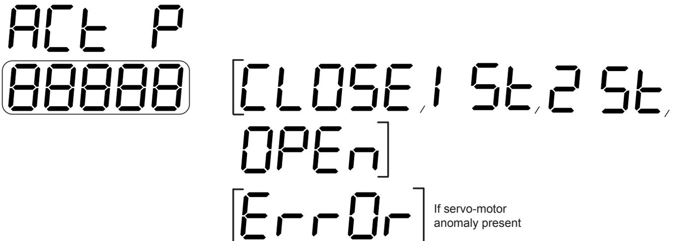
The total opening cycles performed by the servo-motor are also displayed.
