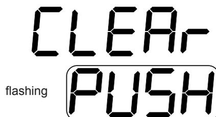
Pressing the key again during this display determines the reset of all meters relative to burner cycles and the return to first stage functioning cycles display.
